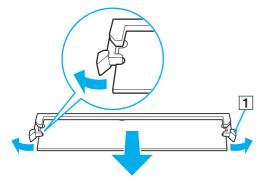
8 Grasp the memory module by the sides and remove from the computer. Store the module in a static-free bag.
